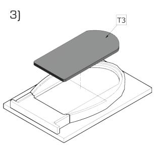
Place the inner plate into the bottom plate cutout.
