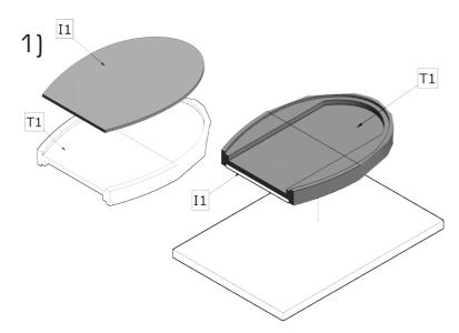
Using a bonding agent, glue the bio-mat (part I1 rear bottom according to the cutting plan of the bio-mat) to the bottom cutout of the bottom rear plate, place the plate by this bottom side with the bio-mat to a stand.
