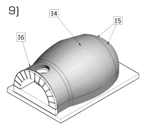
Cover the assembled arch with at least 1 layer of aluminium foil. Place the isolation bio-mat on the aluminium foil according to the cutting plan for the bio-mat. Make sure the bio-mat doesn't get distorted during the application.
