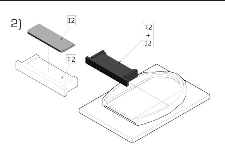
Using a bonding agent, glue the bio-mat (part I2 front bottom according to the cutting plan of the bio-mat) into the bottom cutout of the bottom front plate, place the plate by this bottom side with the bio-mat to the stand
