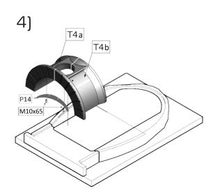
Place the front arch on the front plate of the bottom.
