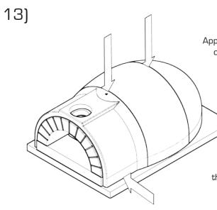
Apply silicone caulk between the body parts and along oven circumference between the bottom edge of the body and the stand - into the formed joint, the used dilatation pads should also get fixed. Silicone the chinks in the way the silicone caulk could be removed in the case of necessity of disassembling the oven (e.g. in the case of a warranty claim).
